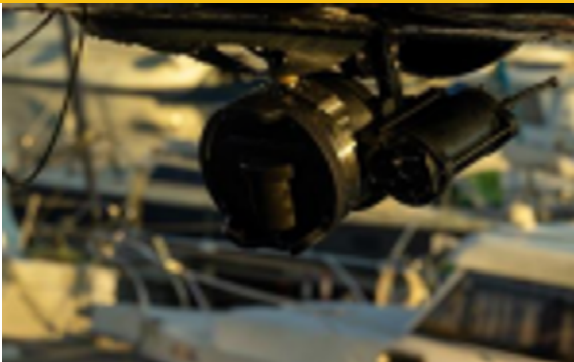
Figure 9 - Kongsberg's M3 HF MBES installed in the PORTUS Autonomous Surface Vehicle.
